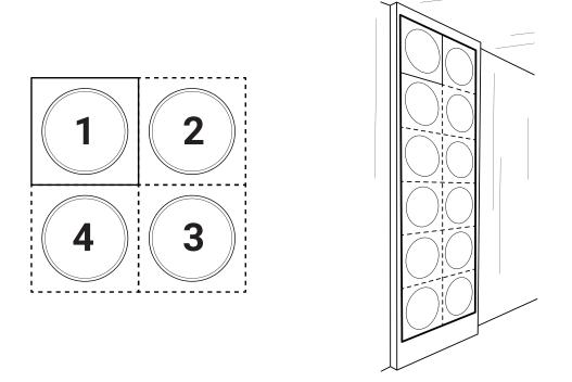
After the first panel is fixed, the adjacent panel is easily positioned to the previous.
