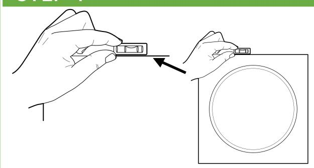
Use a bubble level and put it on top of the wall panel and position with your other hand the panel until the bubble is centered between the two lines.
