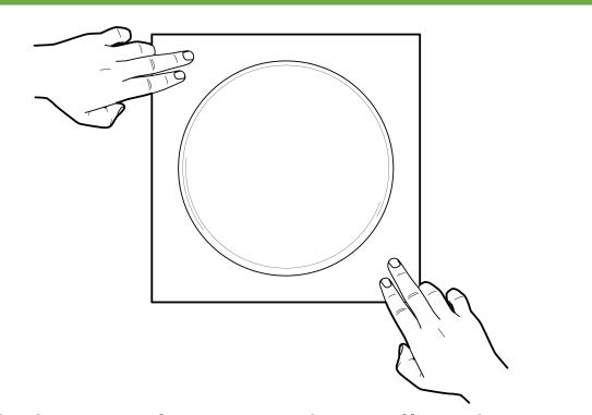
Stick the panel against the wall and press for 5 seconds on the tape joints to the wall.
