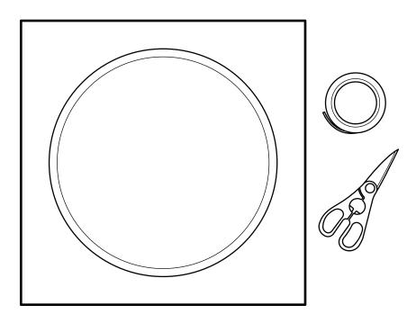
The double sided tape is cutted (with a scissor) and is mounted on the back of the wall panel.
